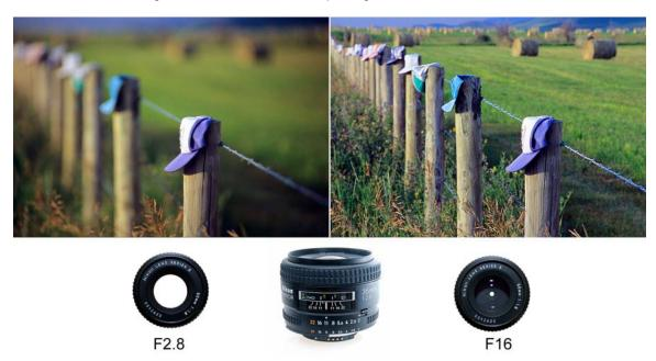
As the lens opening gets smaller the F ratio gets bigger. The largest F-stop on your camera or lens varies, compact cameras might have a maximum aperture of F8 or F11 where an SLR camera lense can have F-stops of F16, F22 or F32. These large F-stops have small openings or apertures and allow the greatest depth of field (see above).
