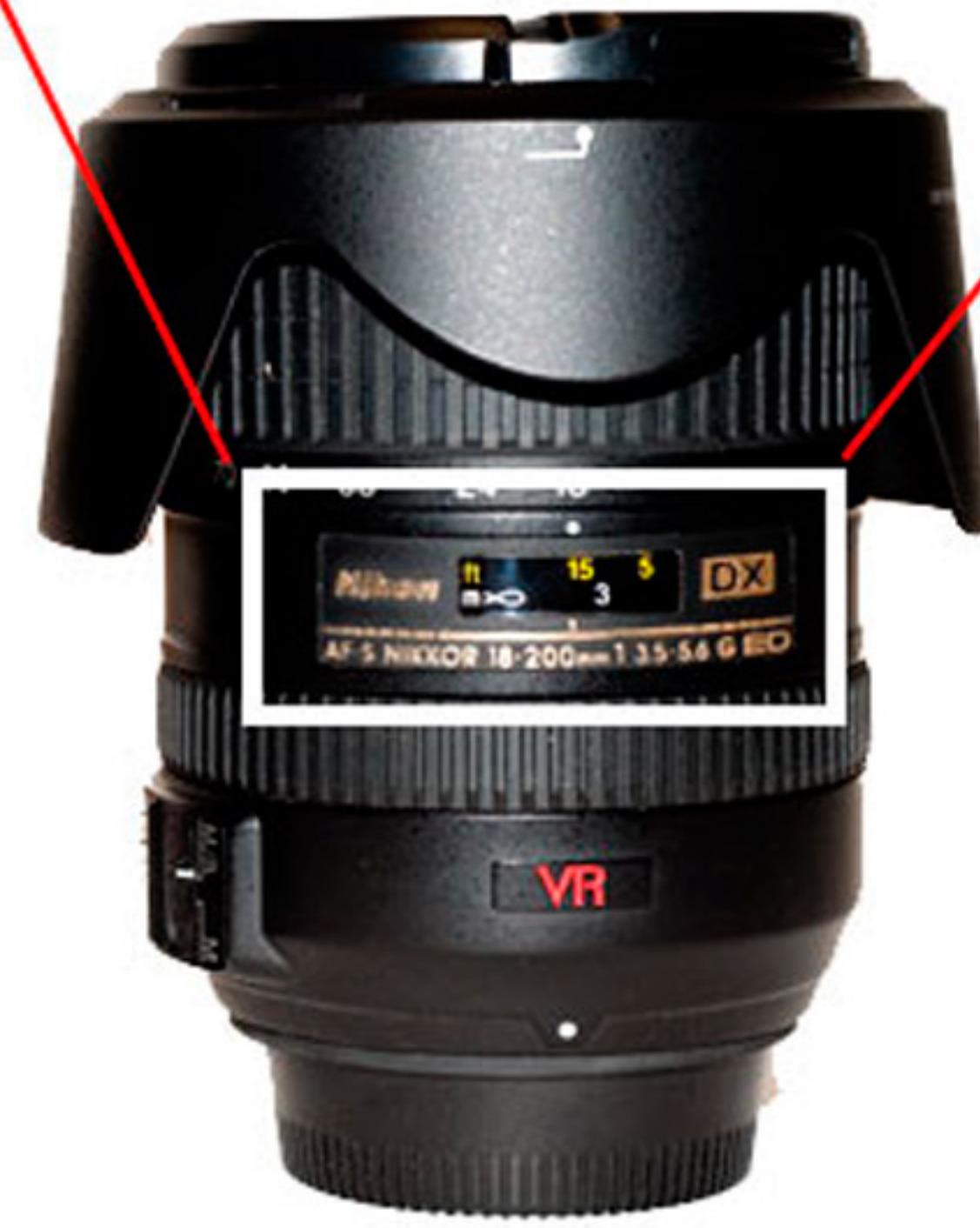
18-200 mm Zoom Lens F3.5-5.6 - widest apture depends on focal length
