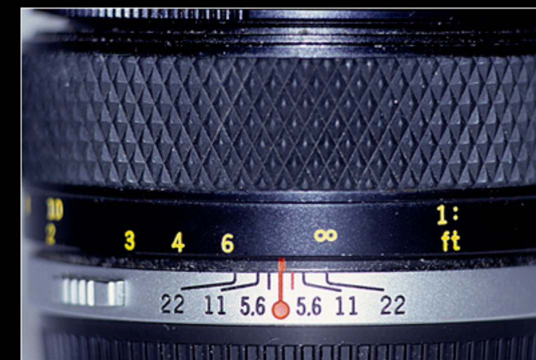
Focus at Hyperfocal distance
